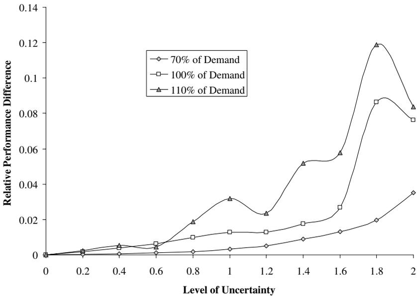
Fig. 4 Relative system performance differences between uniform and optimal allocations (total travel time of uniform minus that of optimal)
