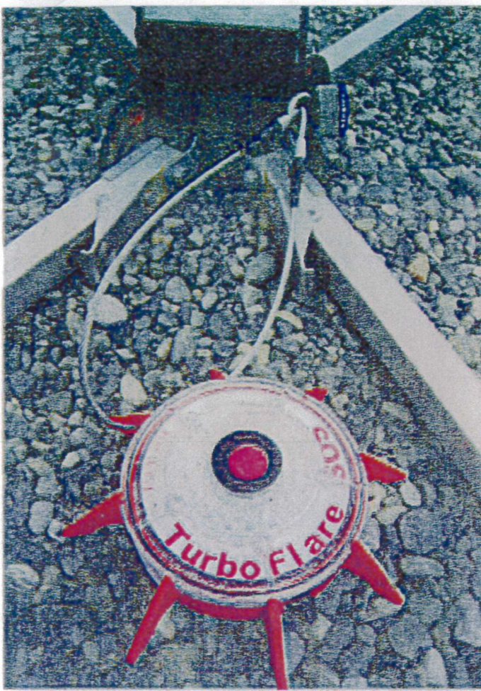
Cable & lock system of Modified turbo flare to prevent theft.
